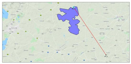
Figure 12. Imagine Broadband microwave radio link passing through the proposed wind farm.
