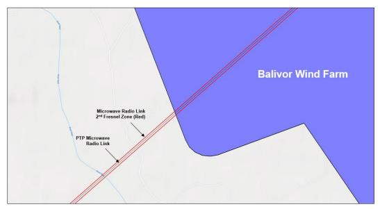
Figure 3. Example of microwave radio link crossing through the proposed wind farm modelled in radio planning software.
