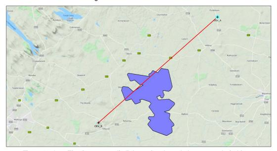
Figure 10. OpenEir microwave radio link passing through the proposed wind farm.
