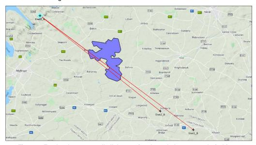
Figure 6. Enet's microwave radio links passing through the proposed wind farm.
