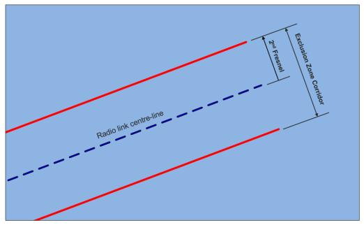
Figure 5. Illustration showing radio link Exclusion Zone
