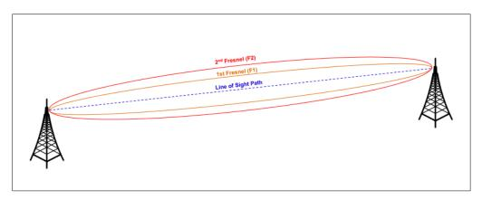
Figure 4. Illustration showing the 1st Fresnel and 2nd Fresnel Zone of a radio link.
