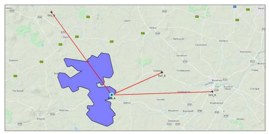
Figure 8. Eir Mobile's microwave radio links passing through the proposed wind farm.
