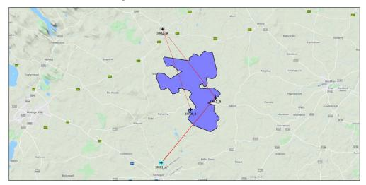
Figure 16. Three Ireland microwave radio links passing through the proposed wind farm.
