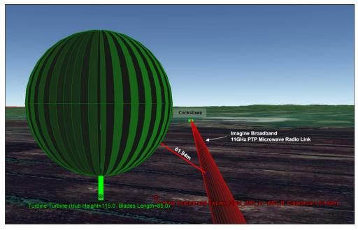
Figure 15. Proposed Turbine relative to Imagine BB Radio Link – 3D View
