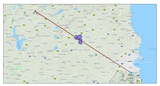
Figure 21. 2RN's radio link passing through the proposed wind farm.
