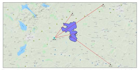
Figure 18. Vodafone Ireland microwave radio links passing through the proposed wind farm.
